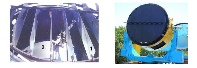
Fig. 1. Solar power plant for studying of thermokinetics of reactionary interaction in obtaining of alloy on the basis of niobium: 1 − sun louver; 2 − paraboloid reflector Ø 2 m
